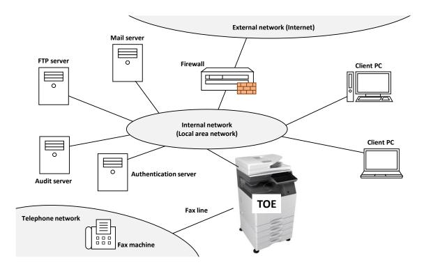
Figure 4-1 Operational Environment of the TOE
