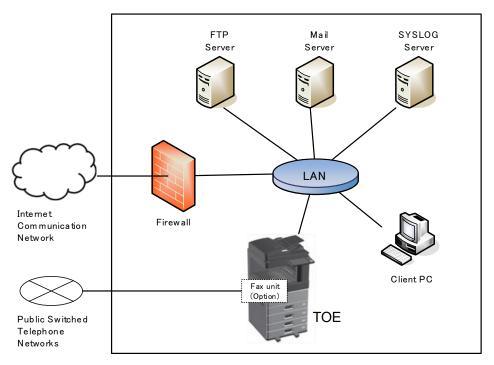
Figure 4-1 Operational Environment of the TOE
