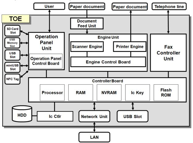
Figure 2 : Hardware Configuration of the TOE
