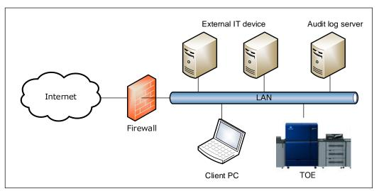
Figure 4-1 Operational Environment of the TOE
