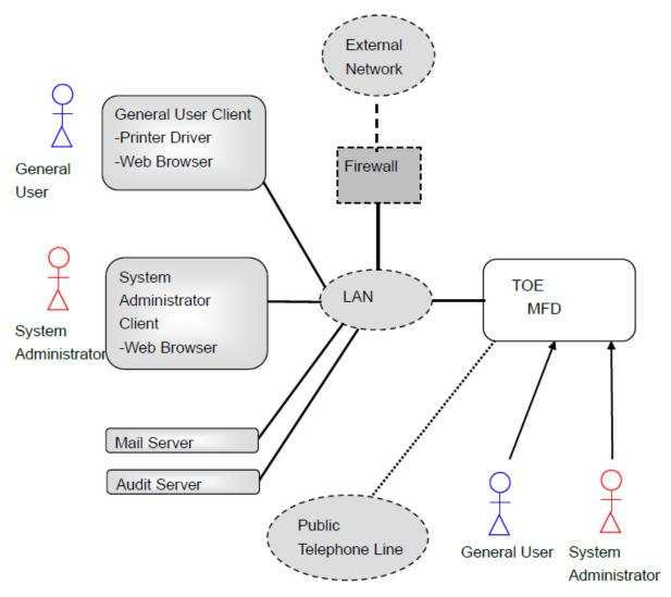
Figure 4-1 Operational Environment of the TOE
