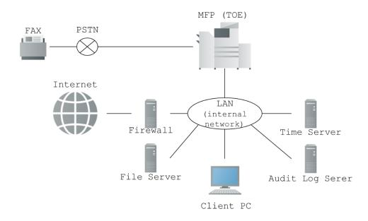
Figure 4-1 Operational Environment of the TOE
