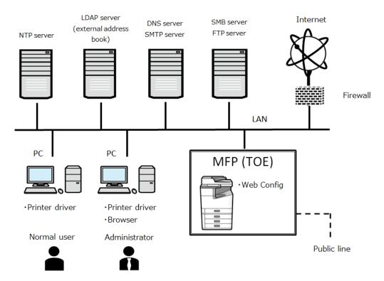
Figure 4-1 Operational Environment of the TOE
