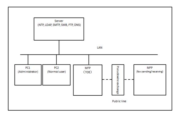
Figure 7-1 Configuration of the Developer Testing
