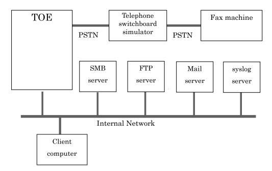
Figure 7-1 Configuration of the Developer Testing
