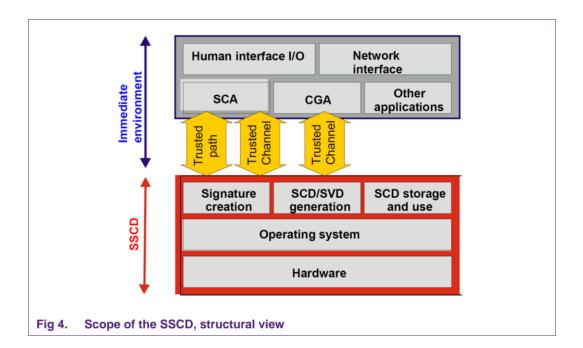
Fig 4 shows the PP scope from the structural perspective. The SSCD, i.e. the TOE, comprises the underlying hardware, the operating system (OS), the SCD/SVD generation, SCD storage and use, and signature-creation functionality. The SCA and the CGA (and possibly other applications) are part of the immediate environment of the TOE. They shall communicate with the TOE over a trusted channel, a trusted path for the human interface provided by the SCA, respectively.
