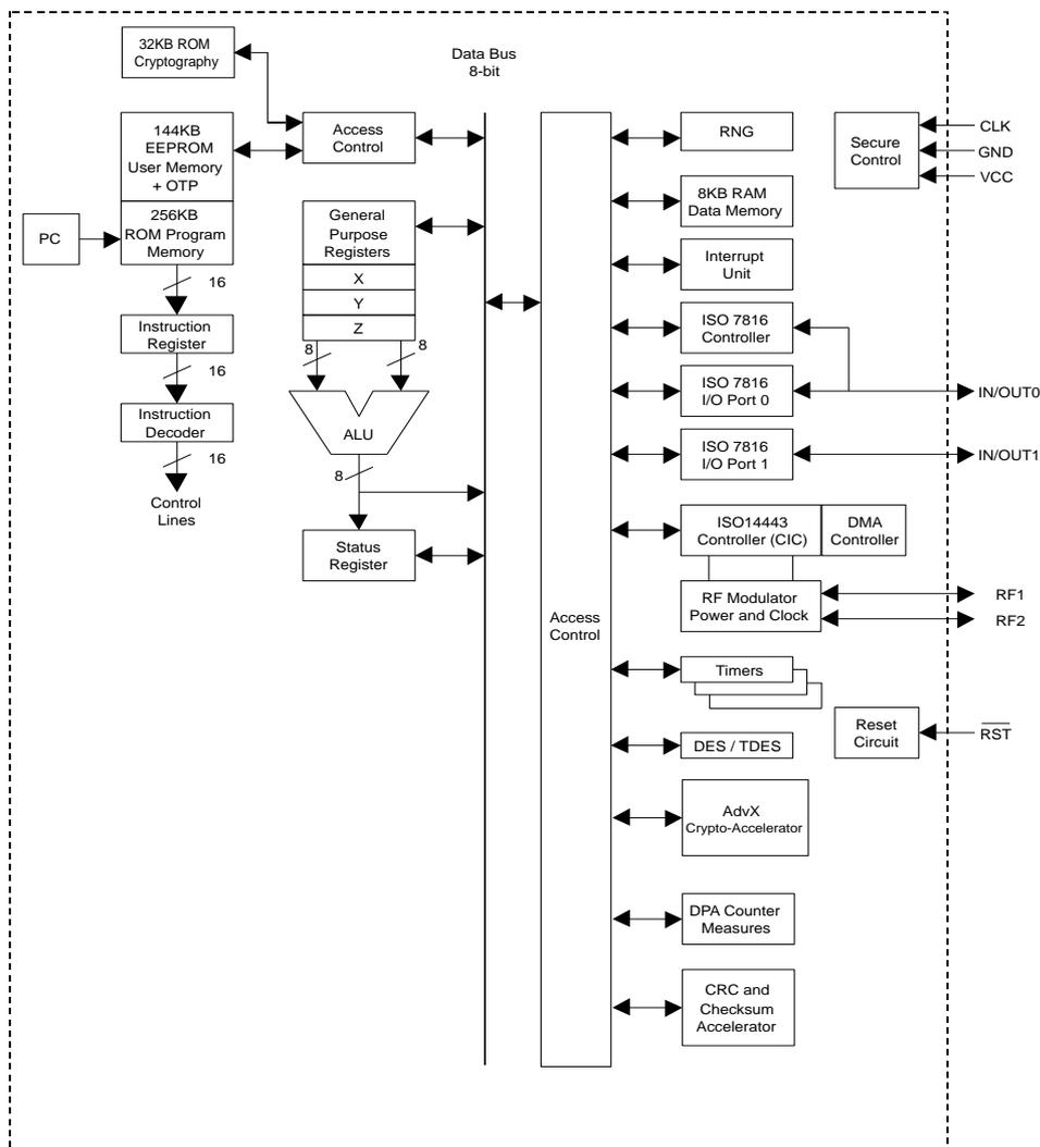
Figure 2-1 AT90SC256144RCFT / AT90SC25672RCFT Block Diagram
