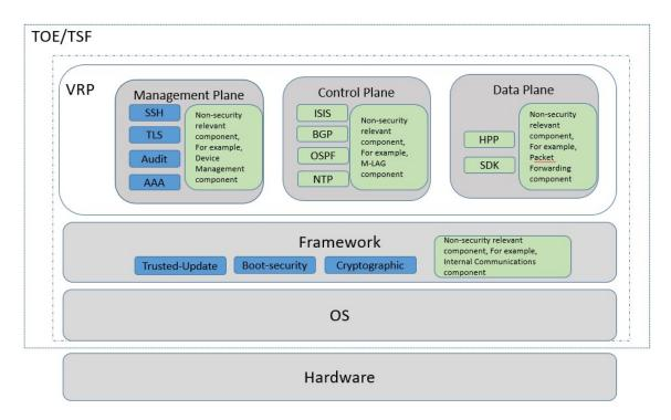
The diagram above describes which modules of the VRP software are part of the TSF and which ones are not. Only the parts of the TOE highlighted in blue implement the SFRs.
