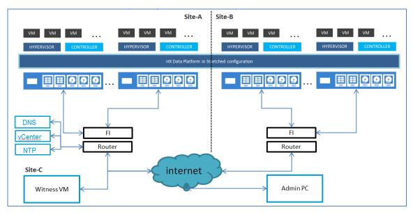
Figure 2 TOE test configuration overview (Site A, Site-B, and Site-C are located in the same location).
