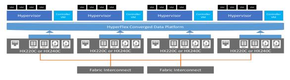
Figure 1. Logical architecture of the TOE.
