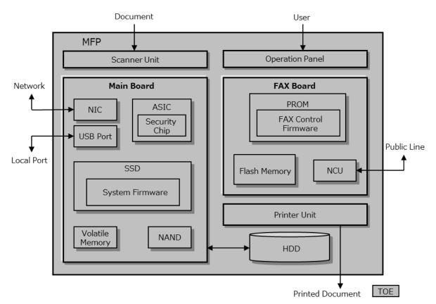
Figure 1-2 Physical Configuration of TOE
