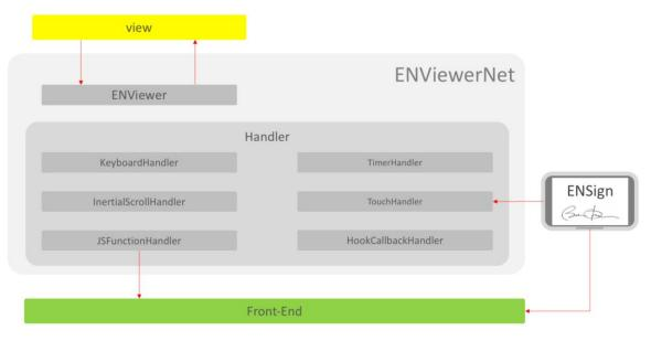
Figure 3 internal design of ENViewerNet process plugin with all handlers
