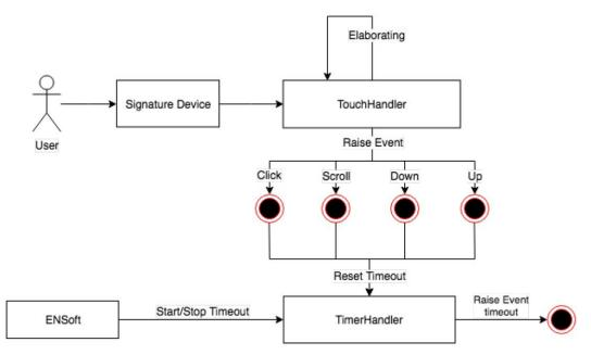
Figure 4 sequence diagram of the user interaction (touch) and timeout handler
