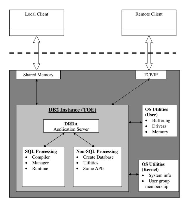
All other functions are allocated to the IT Environment, which in this case is the Host Operating System (OS), inside the darkly shaded box. The DB2 software is tightly linked to the OS and in some cases, security functions are allocated to the OS, as appropriate. For the purposes of this ST, the OS is AIX 5.3, Linux RHEL 4, Linux SLES 9 with SP2, Microsoft Windows Server 2003 Enterprise Edition with SP1, or Solaris 9.
