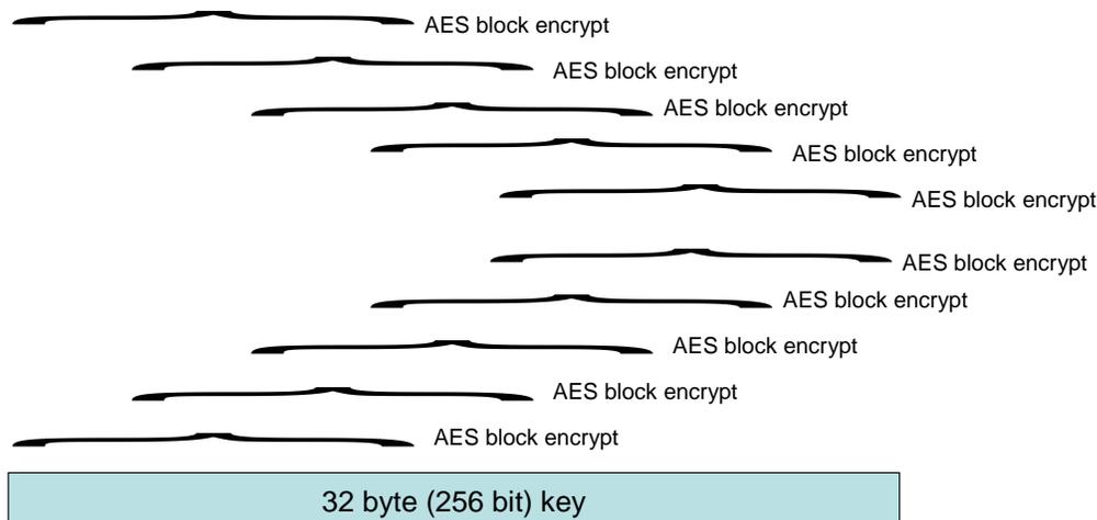
**Figure 7 - Schematic for overlapping ECB encryption**
