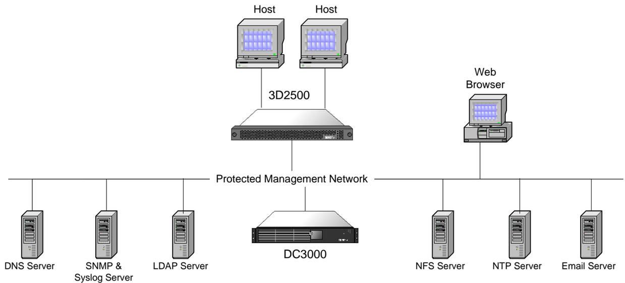
**Figure 4: A DC3000 Defense Center managing a 3D2500 Intrusion Sensor deployed in inline mode (Configuration 2a)**
