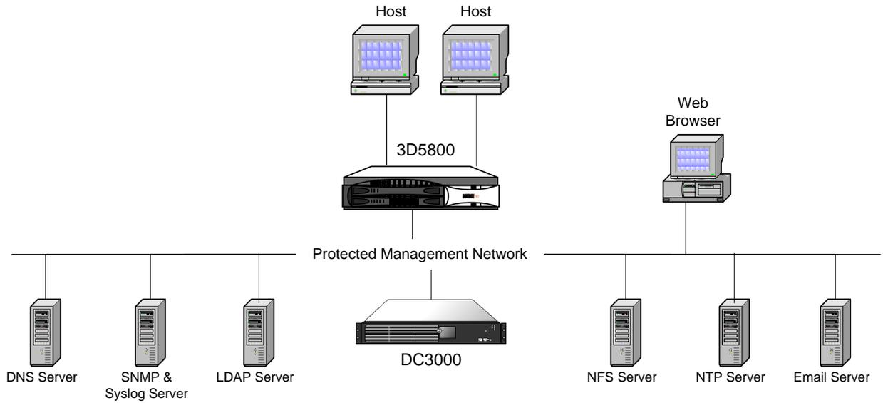
**Figure 9: A DC3000 Defense Center managing a SBLinux Intrusion Sensor deployed in inline mode (Configuration 5)**
