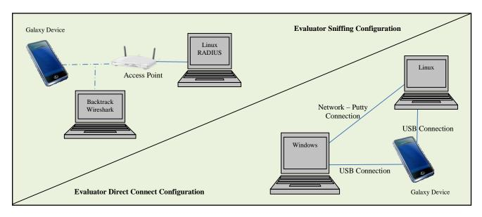
Figure 2 Evaluator Test Setup
