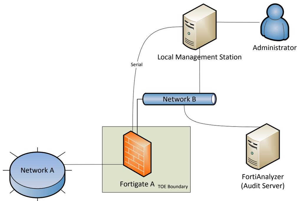
Figure 1 – TOE Physical Boundary
