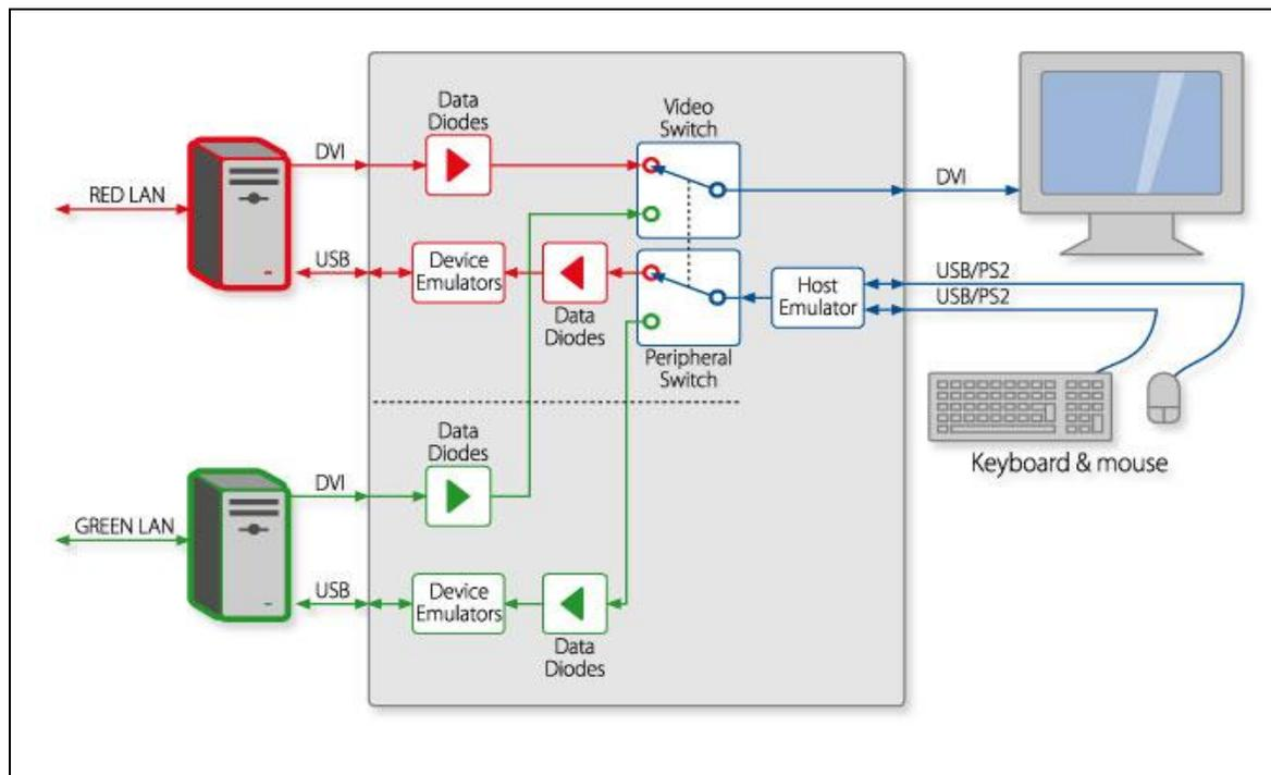
**Figure 7 – Simplified block diagram of 2-Port KVM TOE**
