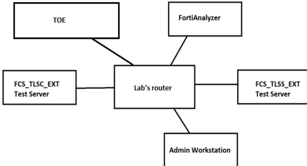
The TOE testing was conducted on the FML-2000E Fortimail Appliance in Gateway Mode. The FortiAnalyzer in the test configuration was used as the audit repository.
