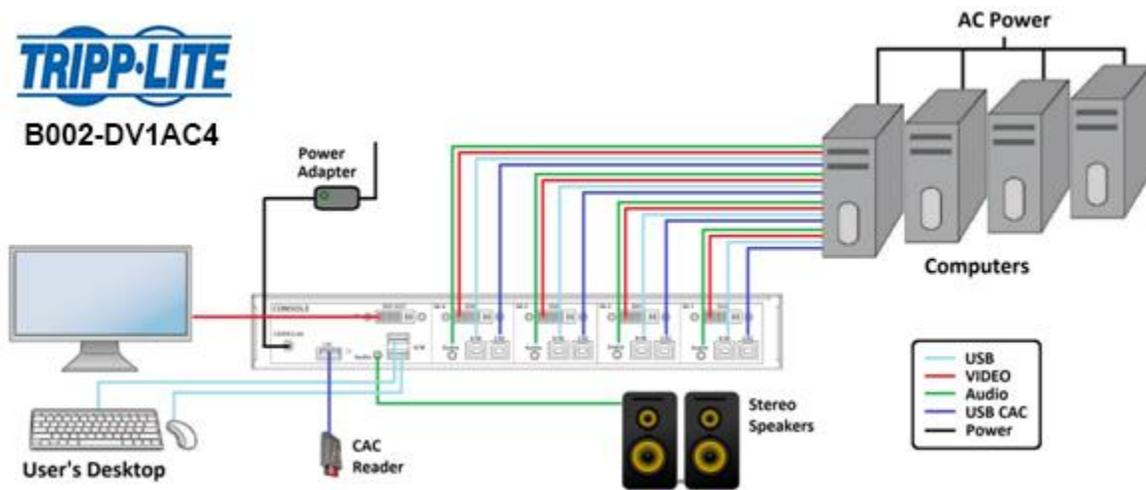
Figure 1: Standard Setup of 4-Port KVM TOE Installation
