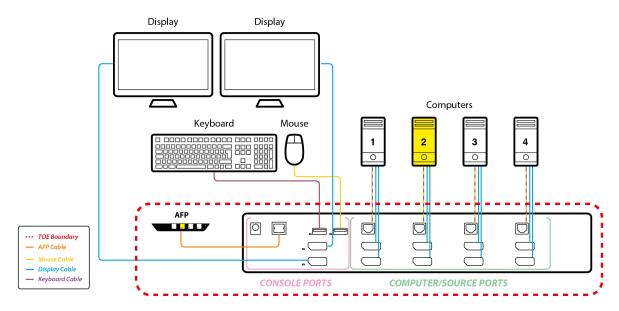
Figure 2 – KVM Switch Evaluated Configuration
