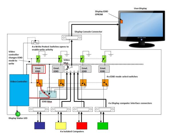
Figure 5 - Display EDID Write Function
