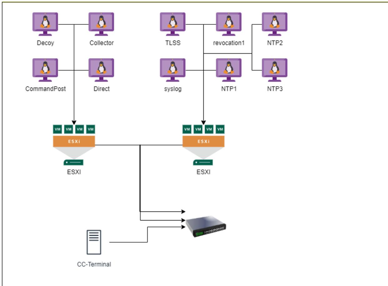
**Figure 3: Virtual Devices Configuration**
