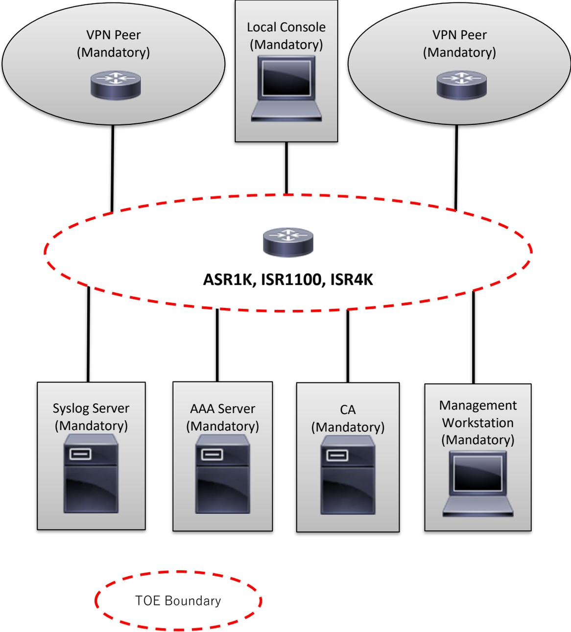
Figure 2 TOE Example Deployment for CSR1000V
