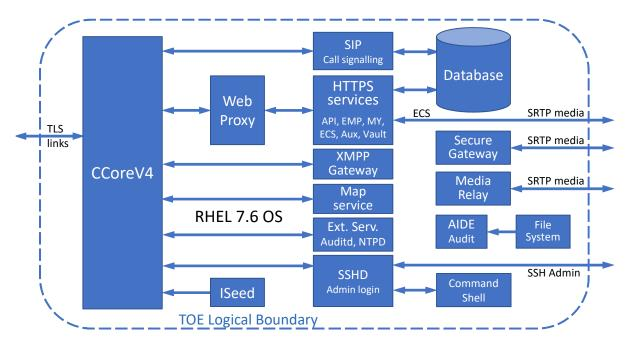
**Figure 1 TOE Software Architecture**
