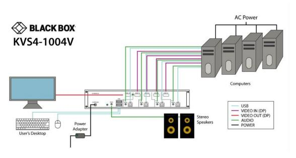
**Figure 1: Setup of 4-Port TOE Installation**
