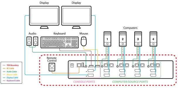
Figure 2 – KVM Switch Evaluated Configuration
