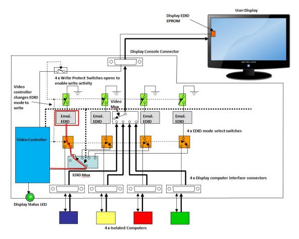
Figure 4 – Display EDID Write Function
