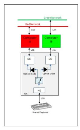
Figure 1 – Simplified Switching Diagram
