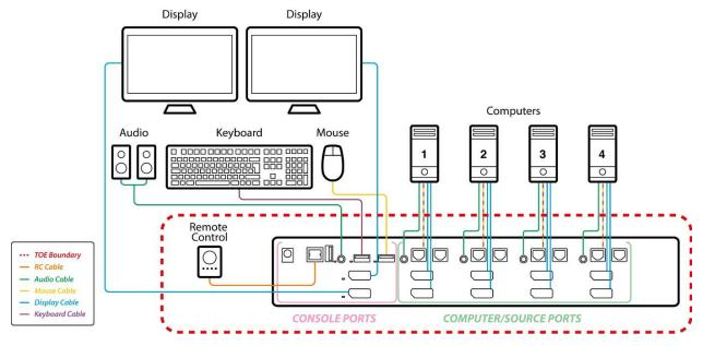
Figure 1: KVM Switch Evaluated Configuration
