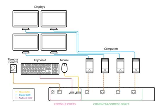
Figure 1 – KM Switch Evaluated Configuration
