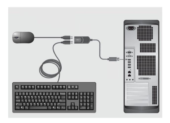
Figure 2 – USB Filter Evaluated Configuration
