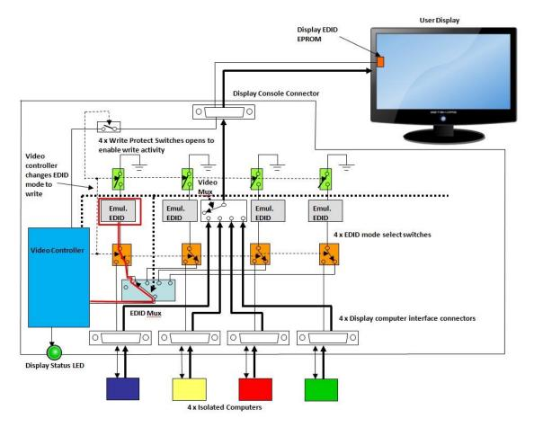
Figure 15 – Display EDID Write Function
