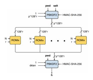
The resulting derived key from this operation is combined with keys chaining to the Application Processor REK and then used to decrypt the FBE DEKs and also to derive the User Keystore Daemon Value.
