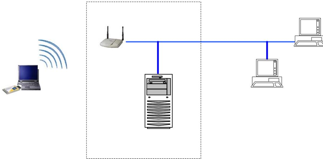
The 3e-WAP accommodates 802.11a/b/g WLAN access and uses Power over Ethernet (PoE) access to the Ethernet WAN to eliminate the need for internal access point power supply units (AC-DC converters) and 110-220V cabling installations. The wireless LANs can include any mobile devices such as handheld Personal Data Assistants (PDAs), mobile web pads, and wireless laptops which support the 802.11a/b/g standards for wireless networking.
