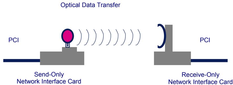
**Figure 1 - High Level view of the Data Diode Interface**
