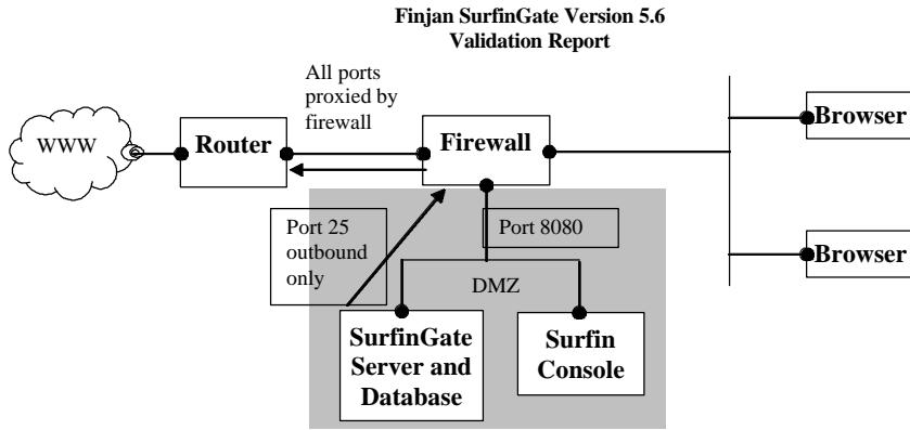
**Figure 2: SurfinGate Evaluated Configuration**
