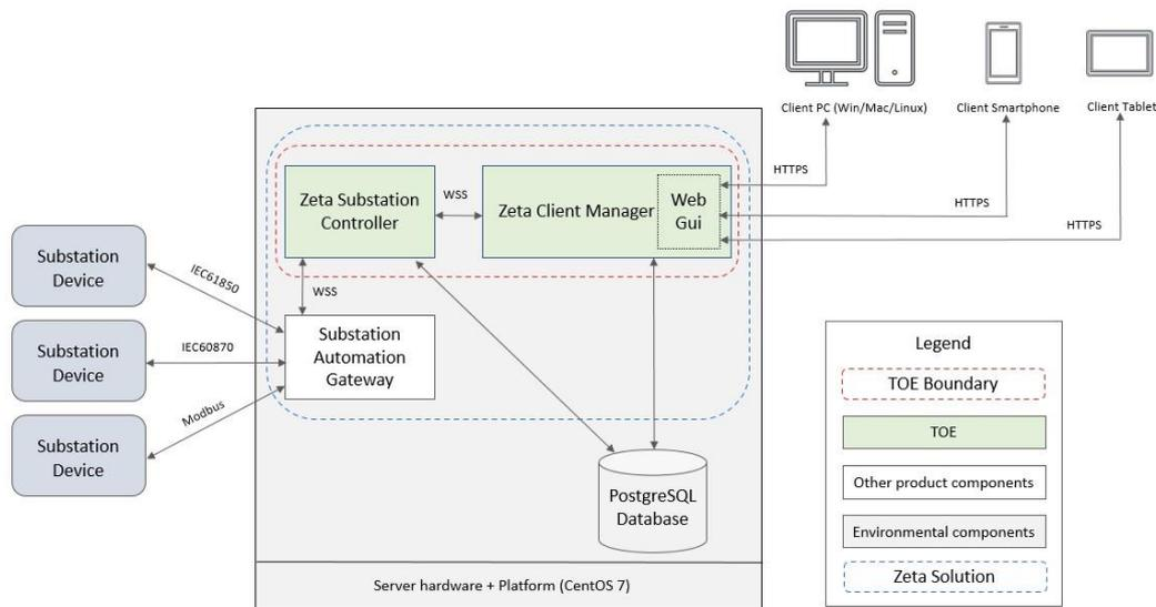
Figure 1 TOE architecture
