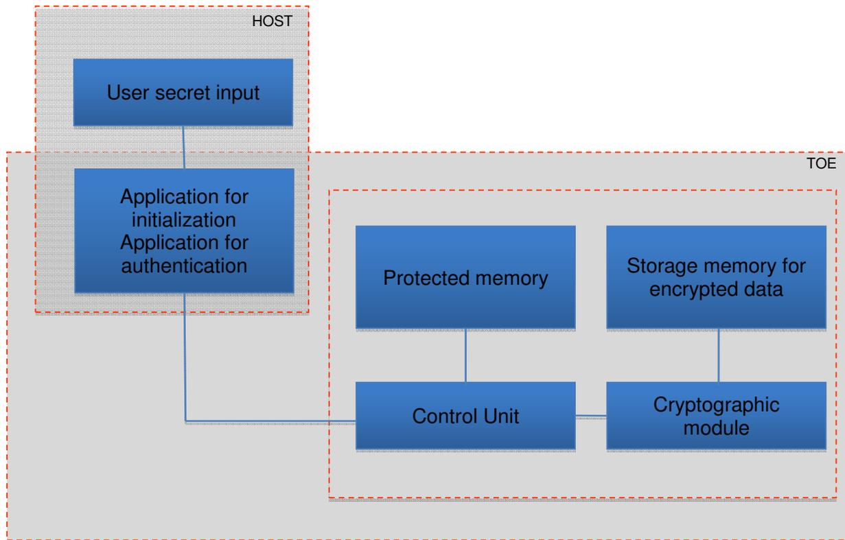
Figure 2 TOE architecture Type B
