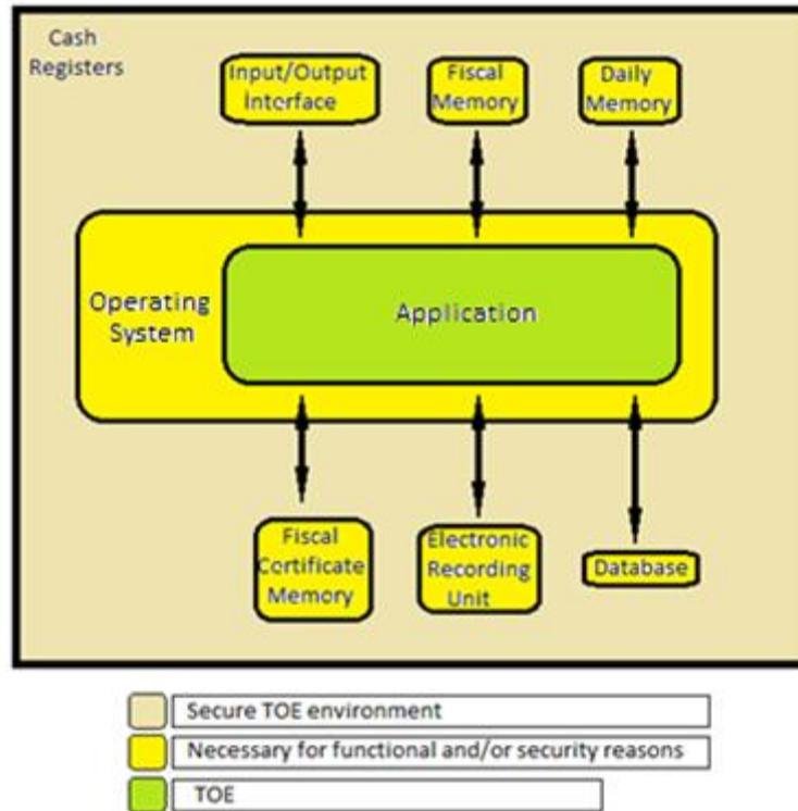
**Figure 1** TOE and related components
