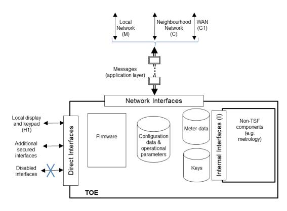
Figure 1 - Generic Smart Meter TOE Architecture
