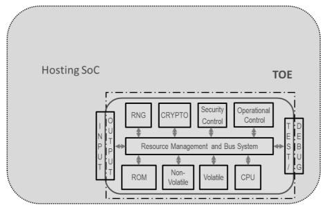
Figure 2: All components are integrated inside the 3S
