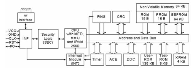
Figure 1: Block diagram of the SLE66CLX640P and SLE66CLX641P
