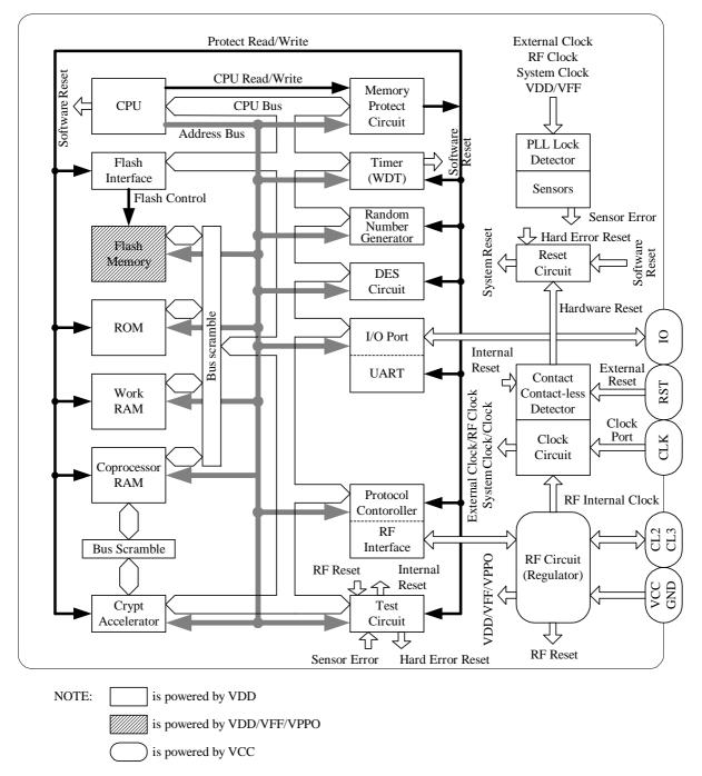
Figure 2-1: Block diagram of TOE
