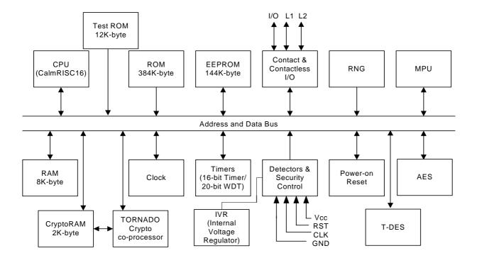
Figure 1. S3CC9GW Block Diagram
