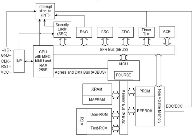
Figure 1: Block diagram of the TOE<sup>1</sup>
