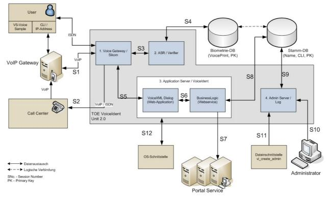
Figure 1: Architecture of the TOE
