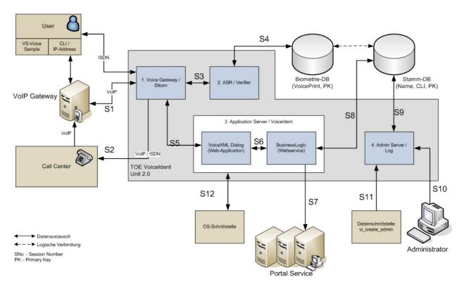
Figure 3: VoiceIdent Unit 2.0 voice verification system
