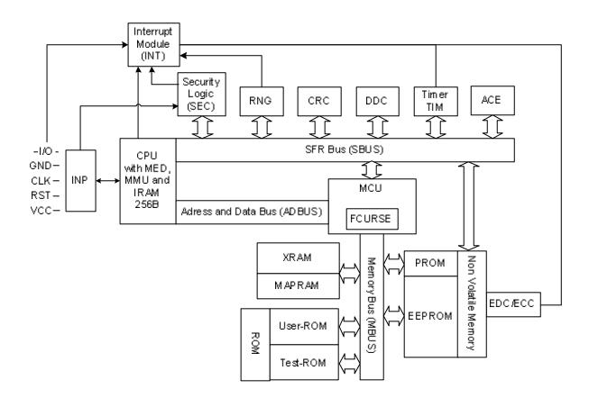
Figure 1: Block diagram of the TOE
