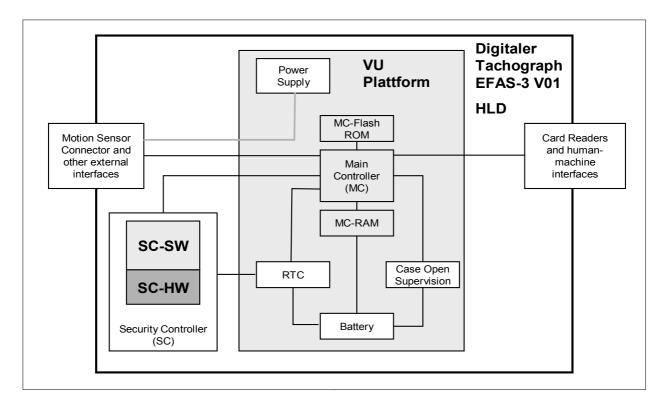
Figure 1: Decomposition of the TOE into its subsystems
