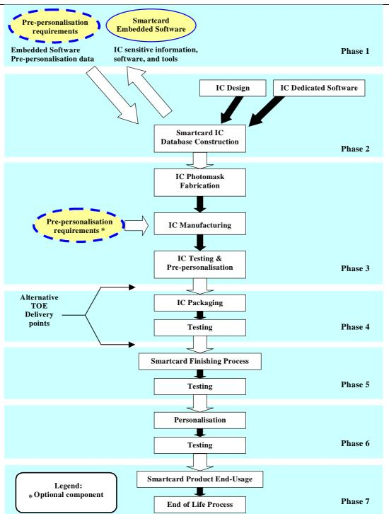
Figure 2-2: Design and Manufacturing Lifecycle
