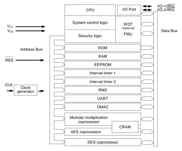
**Figure 2-1: Internal Block Diagram of the TOE**
