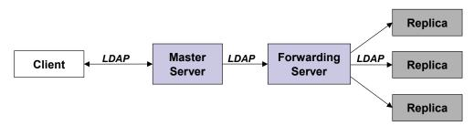
Figure 2: Configuration showing a replication scenario with one master server.
