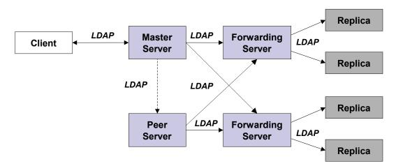
Figure 3: Configuration showing a redundant peer server.
